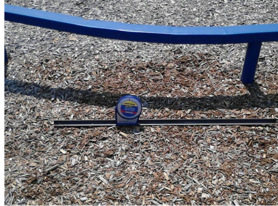
Running slope area needed maintenance. Cross slope was fine.
