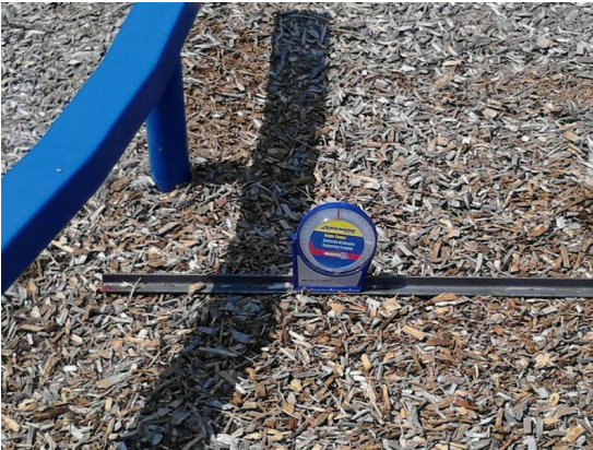
Running slope area needed maintenance. Cross slope was fine.
